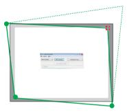
5. Repeat Step 3 and 4 to correct the distortion of the projected image.
