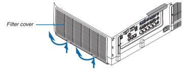
2. Remove the filter unit by pulling out the tab.
