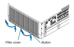
2. Remove the filter unit by pulling out the tab.
