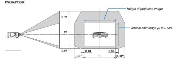
NOTE\*1: Horizontal lens shift range is 0.15H at 150" projected image with the lens NP13ZL
