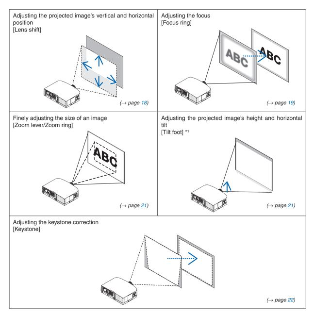
NOTE\*1: Adjust the projected image's height using the tilt feet when you want to project the image at a position higher than the lens shift adjustment range.
