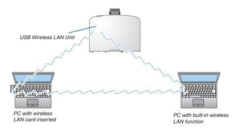
To enable direct communication (i.e., peer-to-peer) between computers and projectors, you need to select the Ad Hoc mode. ( $\rightarrow$  page 123)
