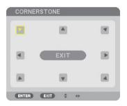
This option allows you to correct trapezoidal distortion. Selecting this item will display the Cornerstone adjustment screen. ( $\rightarrow$  page 32)
