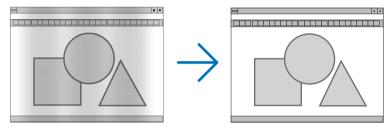
CLOCK ...... Use this item to fine tune the computer image or to remove any vertical banding that might appear. This function adjusts the clock frequencies that eliminate the horizontal banding in the image.
